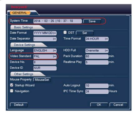
Enter the date (YYYY MM DD) and the time (HH MM SS) in the System Time. Select a Video Standard (NTSC or PAL). Then click OK to save the settings.
